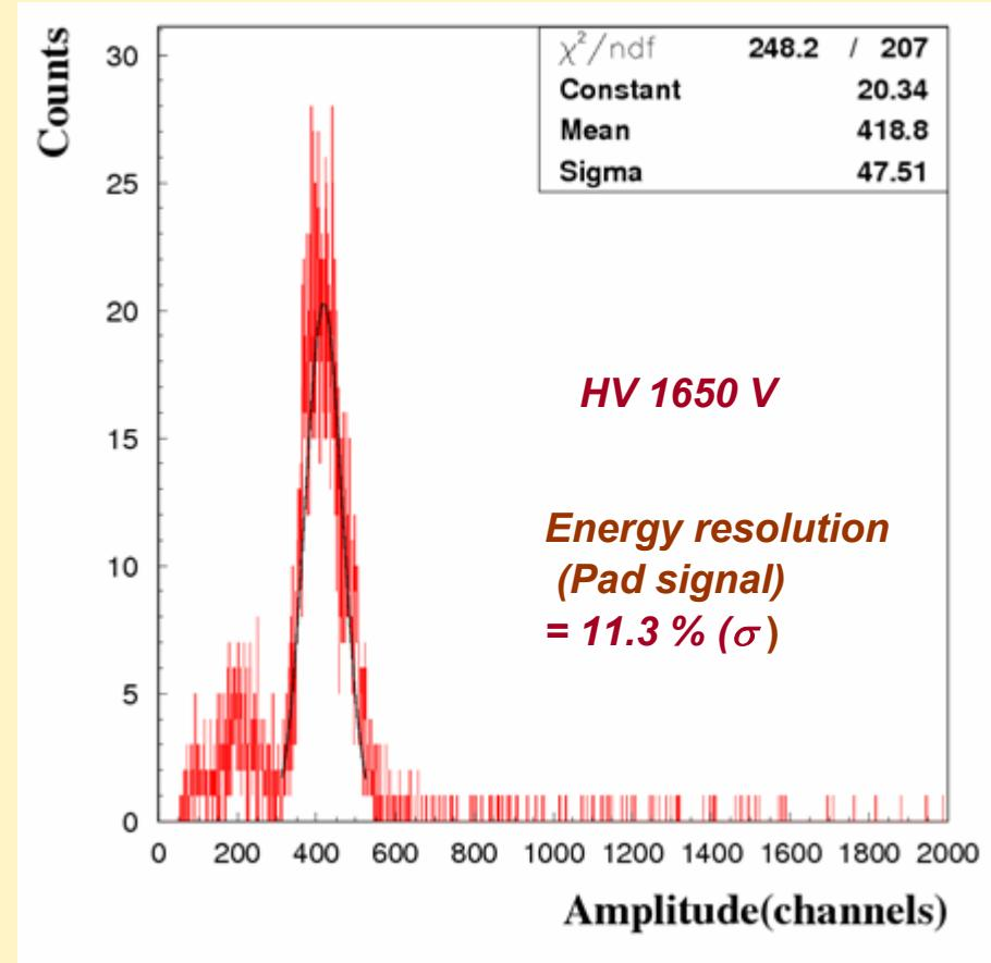
*Readout: PASA (2mV/fC, 1800 e rms) + ADC Converter*
