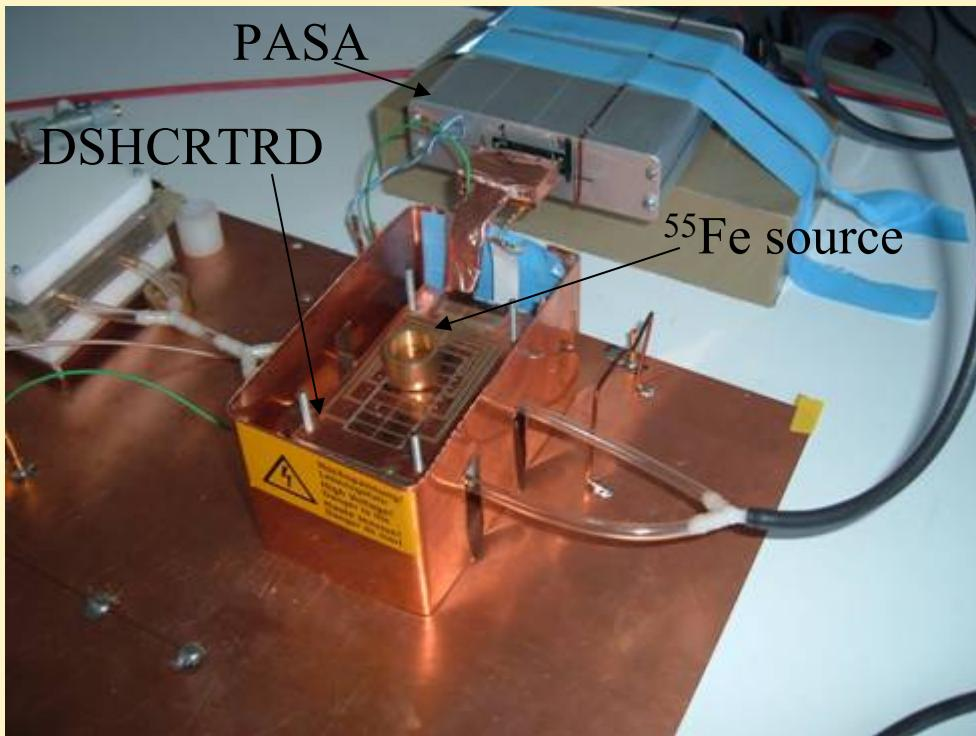
Readout: PASA (2mV/fC, 1800 e rms) + ADC Converter
