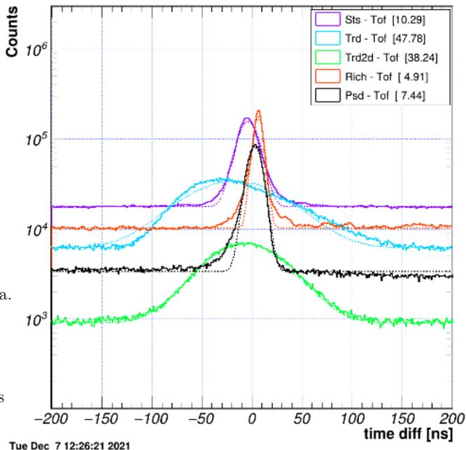
*Time correlation between the data of each mCBM components and a reference selected here to be the ToF system.*
