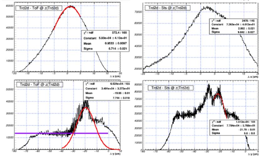
*Spatial resolution in the horizontal ( $\Delta x$ ) direction (upper row) and vertical ( $\Delta y$ ) direction (bottom row) between TRD-2D wrt. the ToF (left) and STS (right) detectors, respectively.*
