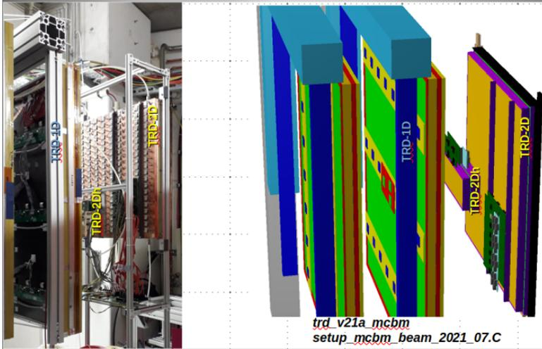
The relative positioning of the TRD-2D prototypes within the mCBM experiment; a picture from the experimental cave (left) and the geometrical setup as used in simulations (right).
