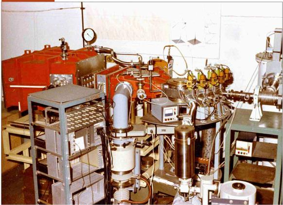
The main components of the DRACULA device were assembled (see left figure) and tested using different radioactive sources in 1986, the beam being not yet transported up to that area.
