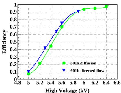
The obtained results, in terms of efficiency (blue symbols) are similar with the results obtained for the previous prototype (green symbols), with gas exchange via diffusion (see the figure above). A similar behaviour as a function of high voltage is observed. A single counter time resolution of 52 ps was obtained.
