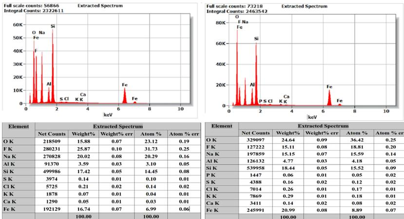
Left-top: electron spectra corresponding to anode surface of irradiated glass; Left-bottom: the corresponding relative elemental composition. Right-top: electron spectra corresponding to cathode surface of irradiated glass; Right-bottom: the corresponding relative elemental composition.
