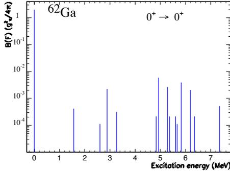
The results, presented in the figure for  $^{62}\text{Ga}$  decay, include both the isospin-symmetry-breaking interactions and shape coexistence and mixing effects. EX-VAM calculations reveal weak decay branches feeding the lowest few excited  $0^+$  states in agreement with recent experimental data.
