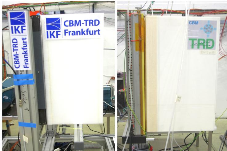
Figure 6.7: Full size radiator prototypes (left: PE hard foam box, right: PMMA hard foam box) for small detector modules.
