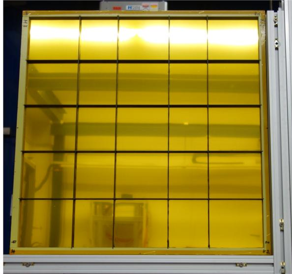
Figure 5.10: Gas foil window supported with the carbon lattice window support structure.
