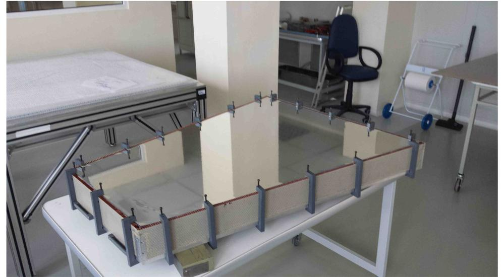
**Tightness test – overpressure flow 6l/hour**
