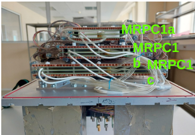
Fig.3 Stacked chambers for cosmic ray test.
