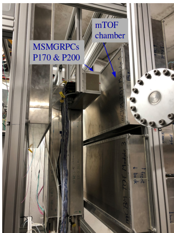
Fig.6 Photo of the box with the prototypes integrated in the experimental setup.
