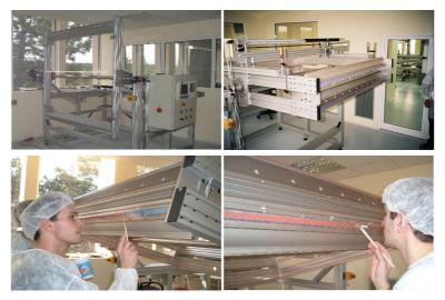
Winding and gluing of multiwire electrodes.
