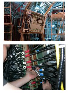
Installing the TRD Super-Modules (SM) in the Experiment
