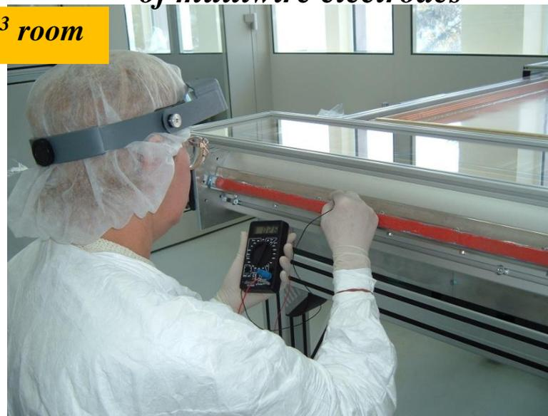
*Final tests: gain uniformity & energy resolution @<sup>55</sup>Fe source*
