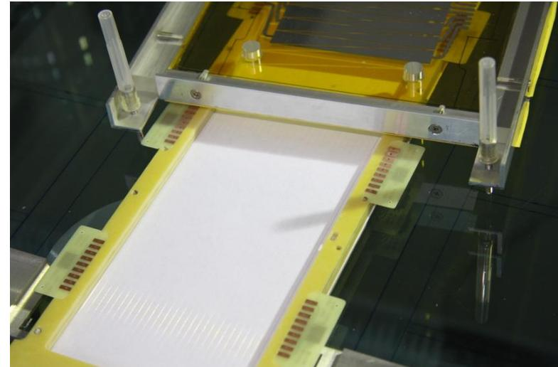
*TRD chamber before to be closed: the readout
