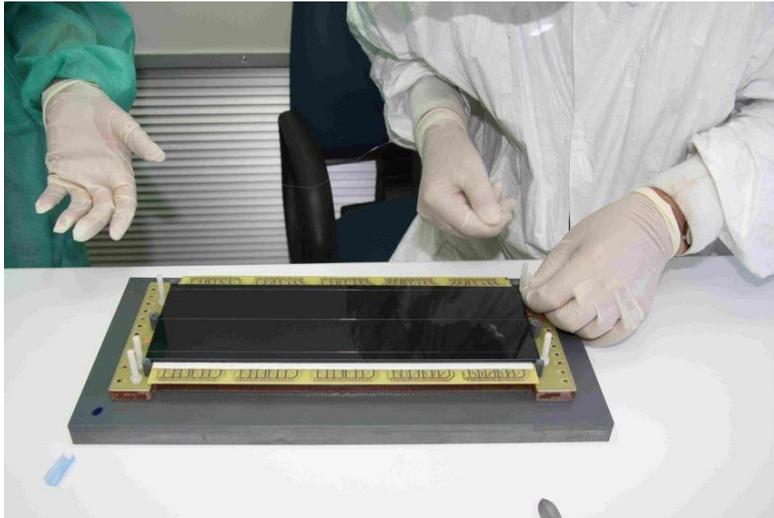
*Stretching the fishing line (spacer)*
