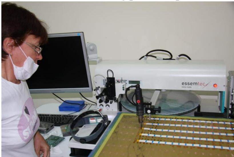
*Assembling of the readout electrode using the vacuum table*
