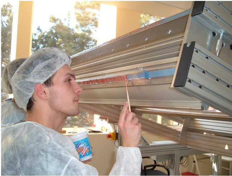
*Pad plane assembling on the vacuum table in 100000 particles/ft<sup>3</sup> room*
