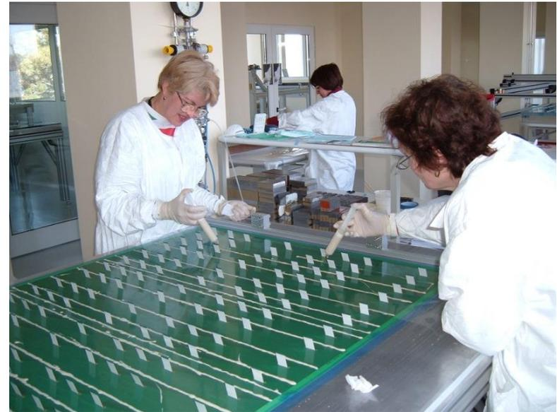
*Soldering of the electrical connections of the multiwire electrodes in 10000 particles/ft<sup>3</sup> room*
