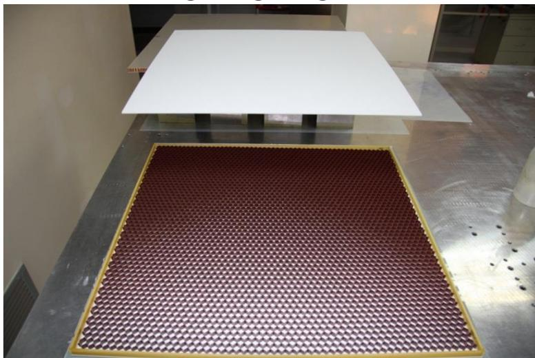
*Gluing & soldering of the multiwire electrodes in 10000 particles/ft<sup>3</sup> clean room*
