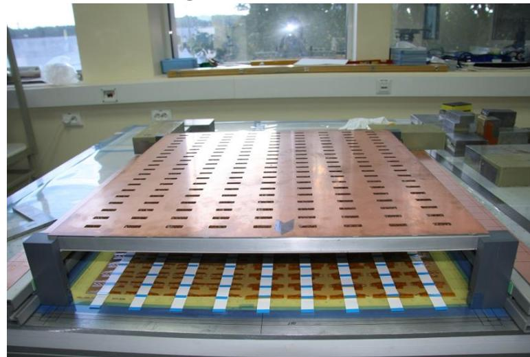
*Assembling of the drift electrode using the gluing table*
