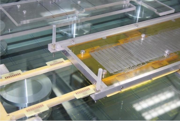
*Gluing of the double-sided readout electrode*
